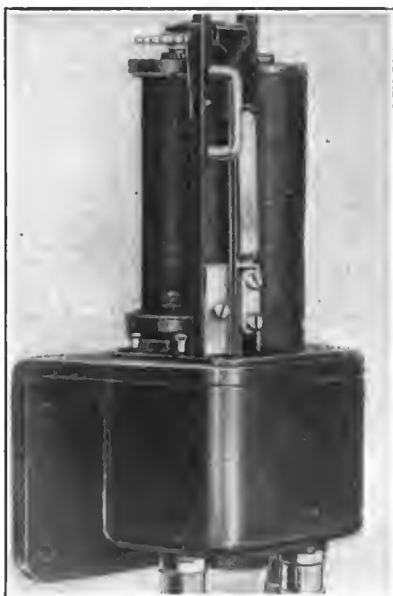
Fig. 3—Delco relay or circuit breaker with cover removed
